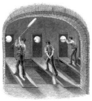
**Fig.6** Cylinder glass making C.1860. Cylinder glass was made by swinging a freshly blown glass bubble so that it elongated by centrifugal force. Both ends of the cylinder were then cut off to form a tube which was then split down one side from end to end and opened out to form a flat, square sheet.
