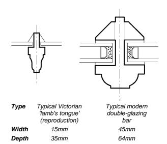
**Fig.8** Modern glazing bar profiles (to the same scale)
