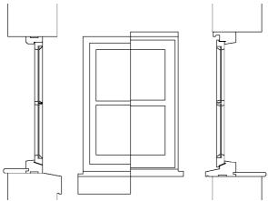
Fig. 11 Casement Windows: The left half illustrates typical Victorian details; the right half illustrates the much larger profiles of a typical modern 'storm-proof' window.
