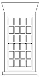
**Fig.2** Early 18th century sash windows. As the price of larger sheets of glass fell, the 'six-over-six' window became common, and the 'four-over-four' (right) was not unknown. After 1709 the windows of buildings in London were required to be set back four inches from the face of the wall, but the box remained exposed. Double hung sashes (with both sashes hung on cords) predominated. From about 1710 to 1730 the segmental headed arch (right) was popular, with both four- and six-paned sashes.
