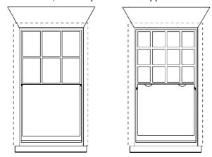
**Fig.10** Left: A Georgian window with its lower sash reglazed. Georgian windows were often reglazed with larger sheets of cylinder or plate glass after 1845. Right: A late 19th century design typical of the 'Queen Anne Revival'. Glazing bar thickness and glazing pattern varied widely. The choice was entirely stylistic and was unrelated to cost or legislation.
