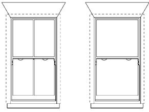
**Fig.9** Late 19th century sash windows with large panes of sheet glass. Notice the short projection of the sides or 'stiles' of the sash below the meeting rail of the upper sash. Known as 'horns', these elegantly shaped projections strengthened the joint where the rail was morticed into the stiles.
