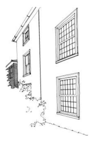
**Fig. 12** Replacement windows (right) contrast sharply with the originals (left) not only in the number of panes but also in their detail. The 'glazing bars' in the double-glazed windows (right) are made of strips of plastic inserted between two sheets of glass and bear no relation to real glazing bars, and the window seems flat and lifeless. It is as if the manufacturers never learned to use their eyes.
