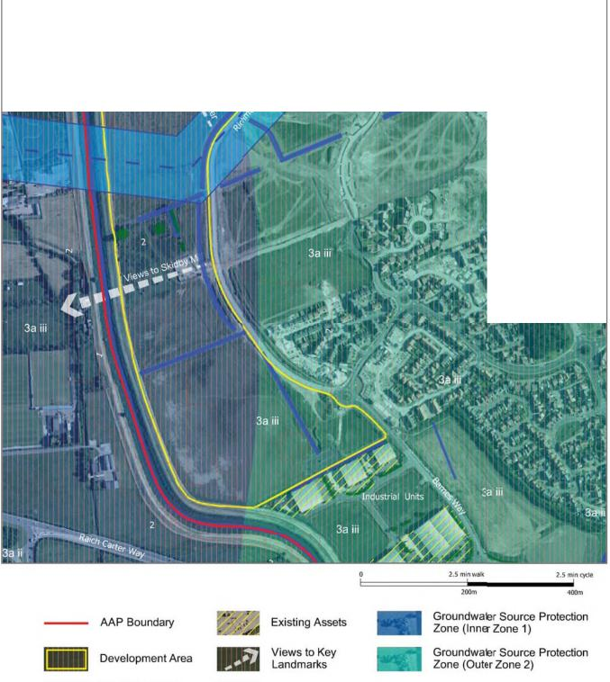
Flood Zone 3a ii 1m Contours (Medium Hazard) Flood Zone 3a iii Mature Trees and (High Hazard) Hedgerows Drains, Watercourses National Grid High Voltage Overhead and Ponds Cable and Pylons with 60m Buffer Zone (not including sewers)
