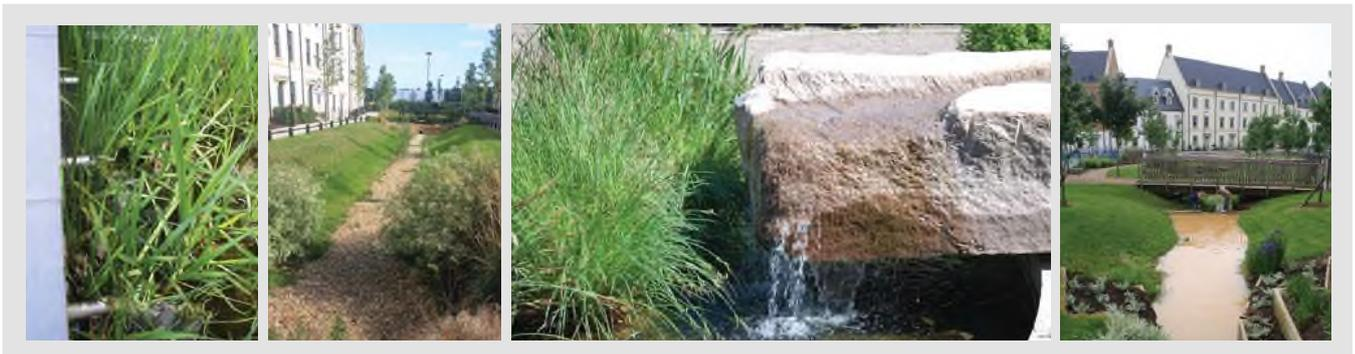
Site controls address run-off near source and include measures such as swales and permeable surfaces
