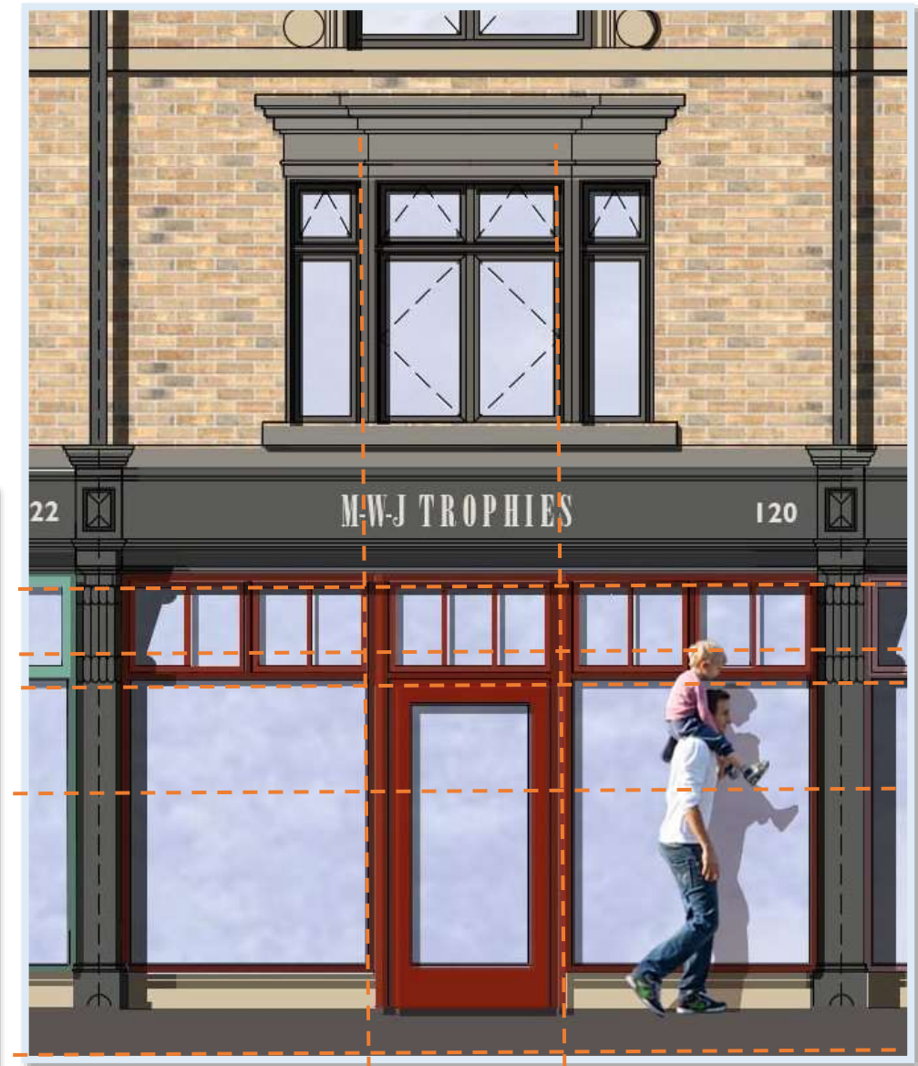
Figure 14 - Illustration showing how the proportions of the various elements of the shopfront should align to create a visually considered design (Author, 2023)
