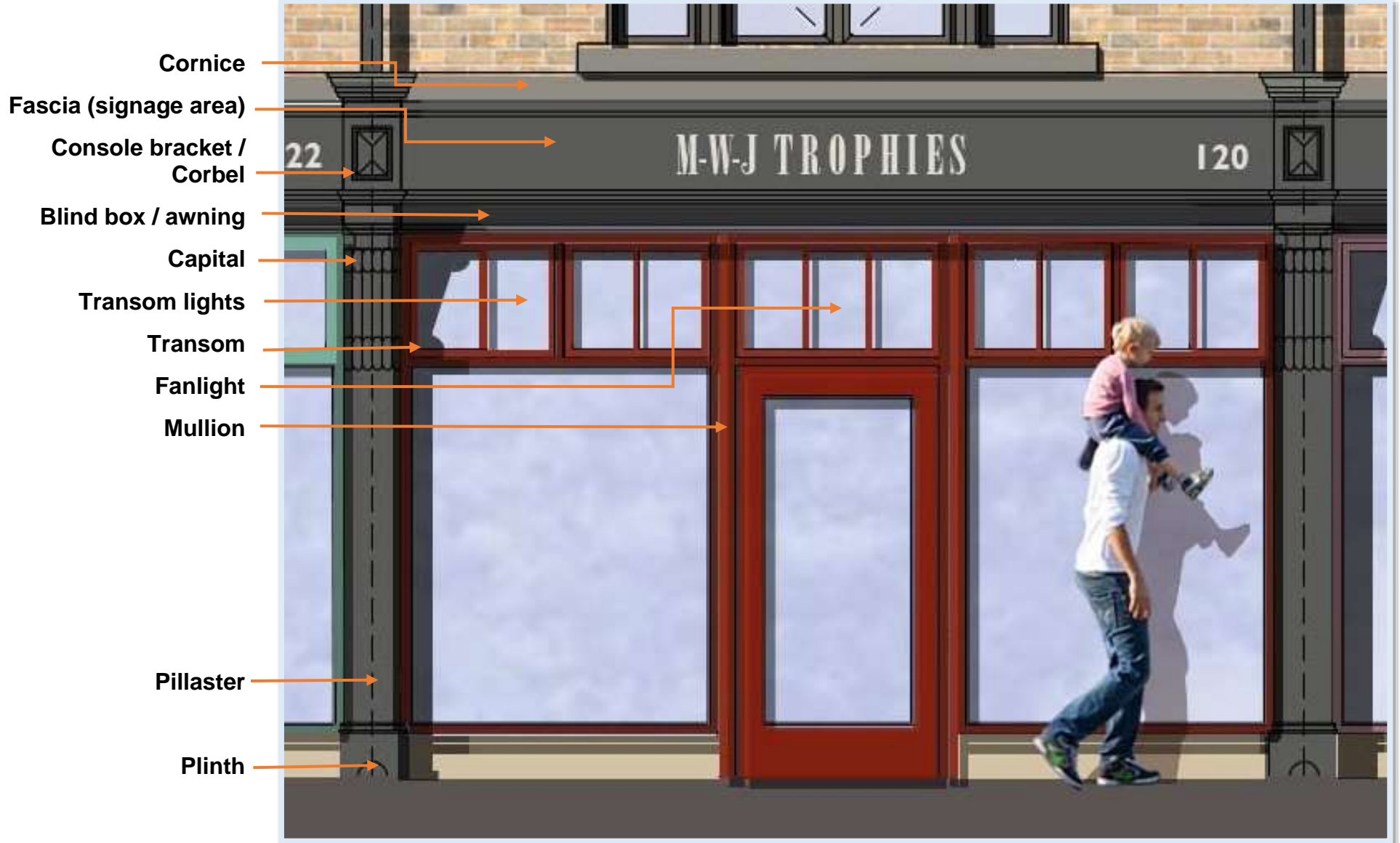
Figure 13 - Illustration showing the various parts of a shopfront design (Author, 2023)
