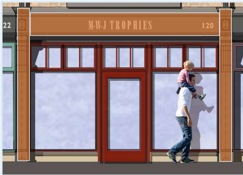
Figure 15 - Illustration showing how the pilasters and fascia frame the shopfront (Author, 2023)
