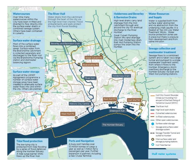
Overview of Hull's water system. (Source: <u>City Water Resilience Assessment - Hull</u> and Haltemprice Water Resilience Profile, Arup,)
