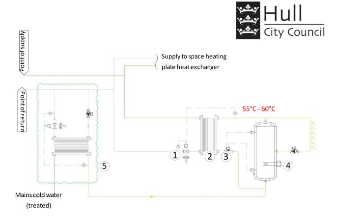
**1. Two-port differential pressure control** – control of supply flow rate and temperatures for each hot water PHE should use two-port variable volume control.
