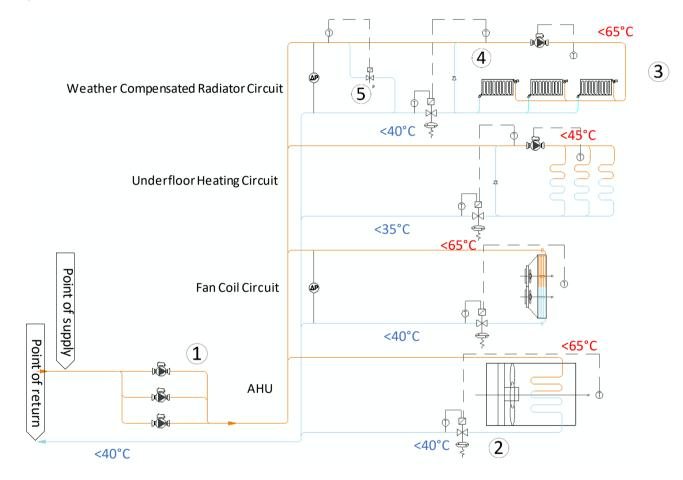
1. Multiple staged variable speed pumps with differential pressure control – secondary system pumps should be controlled to maintain differential pressure across one or more circuit index runs. Using multiple pumps in a parallel arrangement will allow greater range of modulation while maintaining them at their optimum duty point.
