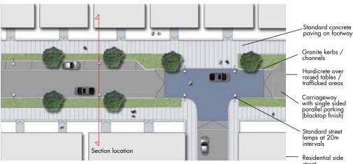
Note: The swatch plan and section are based on a typical street and should be used as a guideline to inform the materials, furniture, layout, character and quality of all the streets within the typology.
