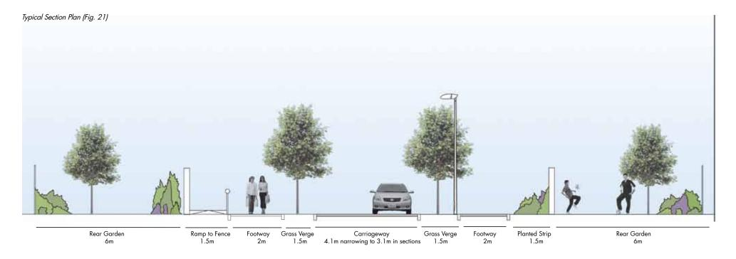
Note: The swatch plan and section are based on a typical street and should be used as a guideline to inform the materials, furniture, layout, character and quality of all the streets within the typology.
