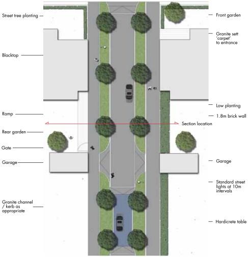
Note: The swatch plan and section are based on a typical street and should be used as a guideline to inform the materials, furniture, layout, character and quality of all the streets within the typology.
