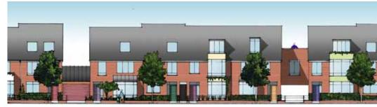
Illustrative Elevation of Typical Residential Type showing continuous built form and breaks every four units. (Fig. 46)
